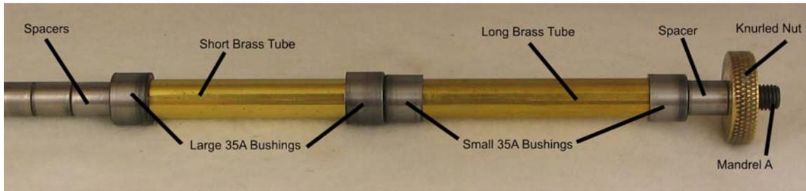
1. Assemble the blanks on the mandrel with the right bushings in the right place. The right bushing can be found by comparing the diameter of the bushing to the piece of hardware that will be placed in that place. For instance, the bushing that is the same size as the clip will fit on the end of the blank that will eventually become the top of the cap.
