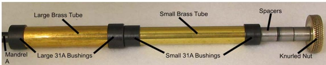
1. Assemble the blanks on the mandrel using the 31A bushings. Select the appropriate bushings for the right place. This can be done by comparing each bushing to the appropriate hardware. The 2 larger bushings are used for the cap blank and the 2 smaller ones are used for the barrel blank.
